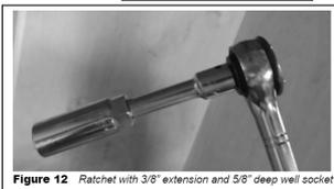
Figure 12 Ratchet with 3/8" extension and 5/8" deep well socket
