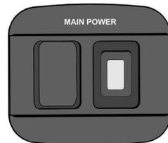
**NOTE:** The combination carbon monoxide/propane alarm requires a constant 12-volt power source. The carbon monoxide/propane alarm remains operational when the battery disconnect solenoid switch, or “main power switch,” is in the “ON” position or when the ignition key is rotated to the “ON” position.
