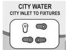
**To disconnect:** Turn off water at the pressurized source first, disconnect hose from the water source, (to release pressure off the system) then disconnect the hose at the city water connection on utility center last.
