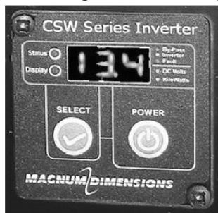
**NOTE:** When in *Inverter Mode* you will be able to cycle through Battery Voltage, Inverter Power, inverter settings and error codes. When in *Bypass Mode* you will be able to cycle through Battery Voltage, inverter settings and error codes. Inverter Power will not be available because the inverter is idle.
